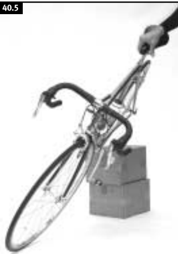
Simulating a very steep head angle to the point of creating negative fork trail and consequent very low stability: When the bike is leaned, the front wheel turns away from the direction of lean to get farther out from under the rider and cause him or her to crash sooner.
