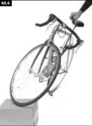
Simulating a very shallow head angle and consequent large fork trail, which imparts great stability: The wheel flops out of the plane of the bike at low lean angles to rapidly get back under the rider's weight and stabilize the rider.
